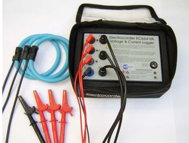
Photo shows ElectroCorder EC664-VA, with Rogowski sensors and voltage leads.
